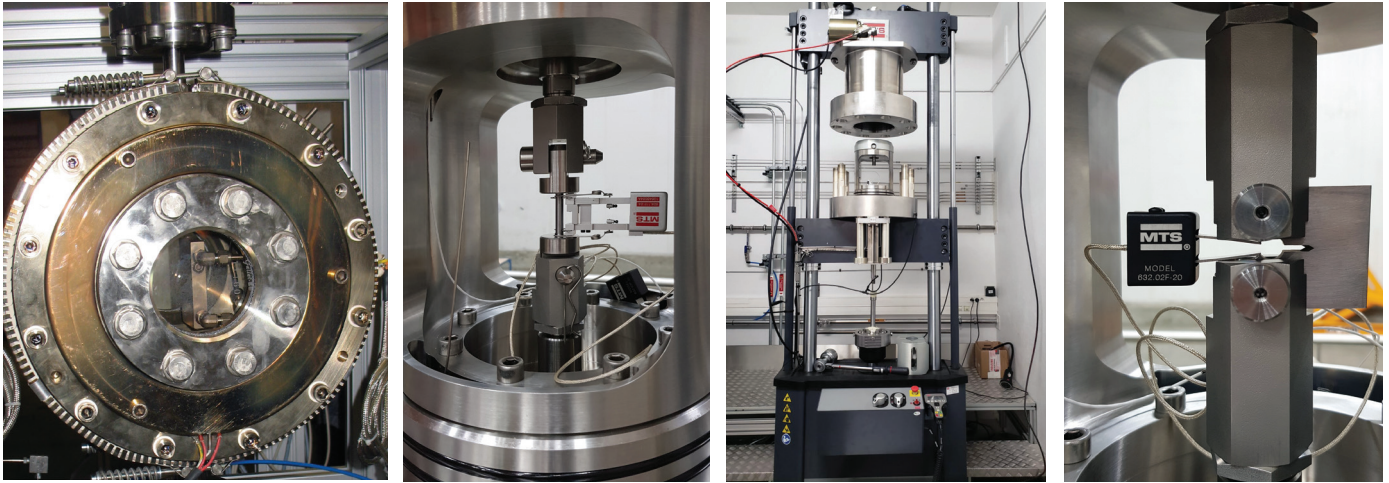
Autoclave with optional optical quality glass window to accommodate non-contacting strain measurement solutions.
